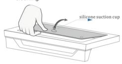
To reinstall the glass panel, simply carry out the above process in reverse, placing the glass panel back into the unit, then using a screwdriver to replace and tighten the oven door screws. **CAUTION!** Always ensure the glass panel is firmly secured and the screws are securely tightened before attempting to close the oven door.
