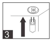
Rotate the light cover counterclockwise to tighten it.
